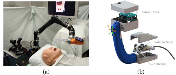
Fig. 8. Robots for intervention and treatment: (a) Kepler Intubation System (McGill University, Canada) [29]. (b) Robotic Endoscope Automated via Laryngeal Imaging for Tracheal Intubation (REALITI, ETH Zurich, Switzerland) [33].
