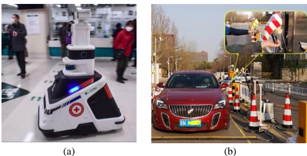
Fig. 3. Robots for screening. (a) A robot used for temperature monitoring at a hospital in Shenyang, China. (b) SHUYU robot developed by the Tsinghua University, China, allows for drive-through rapid temperature screening [13].
